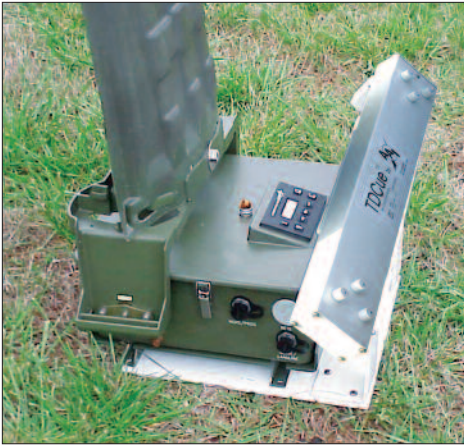
TDCue non-contact hit sensor system, with E-type silhouette
